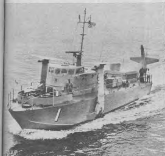
GUNBOAT FLAGSTAFF , built by Grumman, has conventional configuration, two foils forward, one aft
