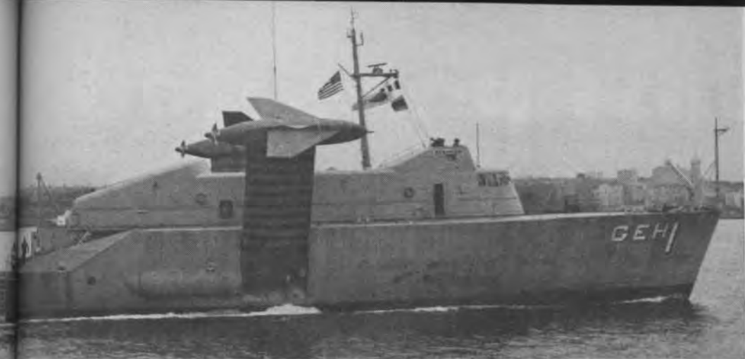
forward and one aft, are in retracted position, displaying their winglike construction. Plainview , the largest hydrofoil ever built, is 212 feet long, displaces 300 tons and is intended to perform the duties of a destroyer
