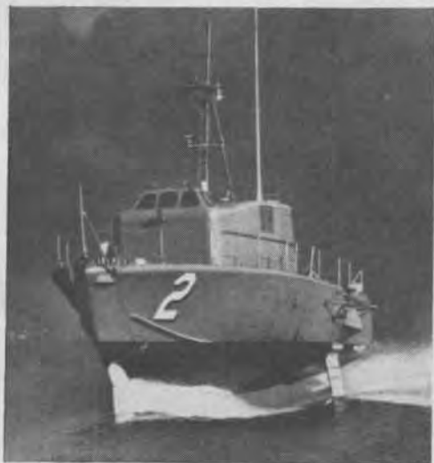
GUNBOAT TUCUMCARI , built by Boeing, features canard configuration, with one foil forward, two aft
